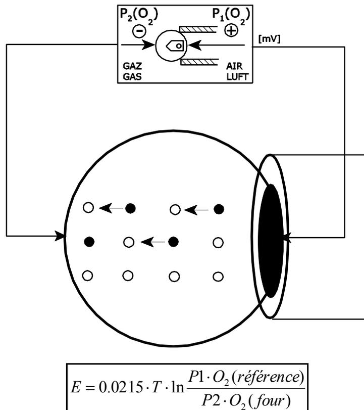
E = tension [mV] aux bornes
