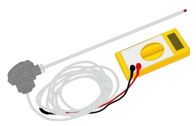
An oxygen probe works by comparing the oxygen level in the kiln with the oxygen level inside the alumina tube. This is why the air inside the tube must always be renewed. If the temperature of the the zirconia tip is over about 700 °C, it produces an electrical voltage. The less oxygen in the kiln, the bigger the electrical voltage, so the voltage can be used as a guide to the oxygen level.
